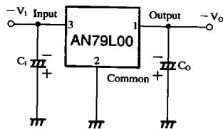
$C_i$  is connected when the input line is long.  $2\mu\text{F}$
