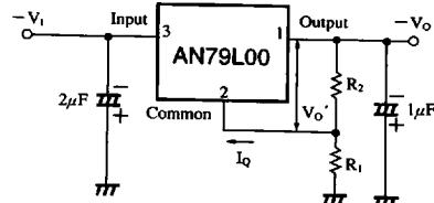
$$|V_{o1}| = V_o \left( 1 + \frac{R_1}{R_2} \right) + I_Q R_1$$
