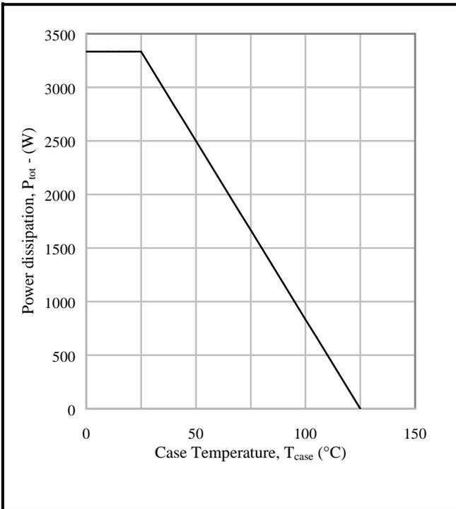
**Fig.5 Power dissipation**
