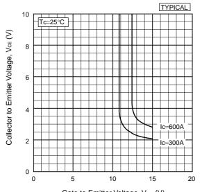
$\label{eq:Gate to Emitter Voltage, Vge} Gate \ to \ Emitter \ voltage, Vge \ (V) \\ \textbf{Collector to Emitter voltage vs. Gate to Emitter voltage}$
