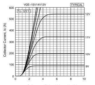
$\label{eq:collector} \mbox{Collector to Emitter Voltage, $V_{\text{CE}}$ (V)$} \\ \mbox{Collector current vs. Collector to Emitter voltage}$
