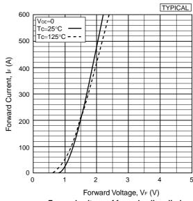
Forward voltage of free-wheeling diode
