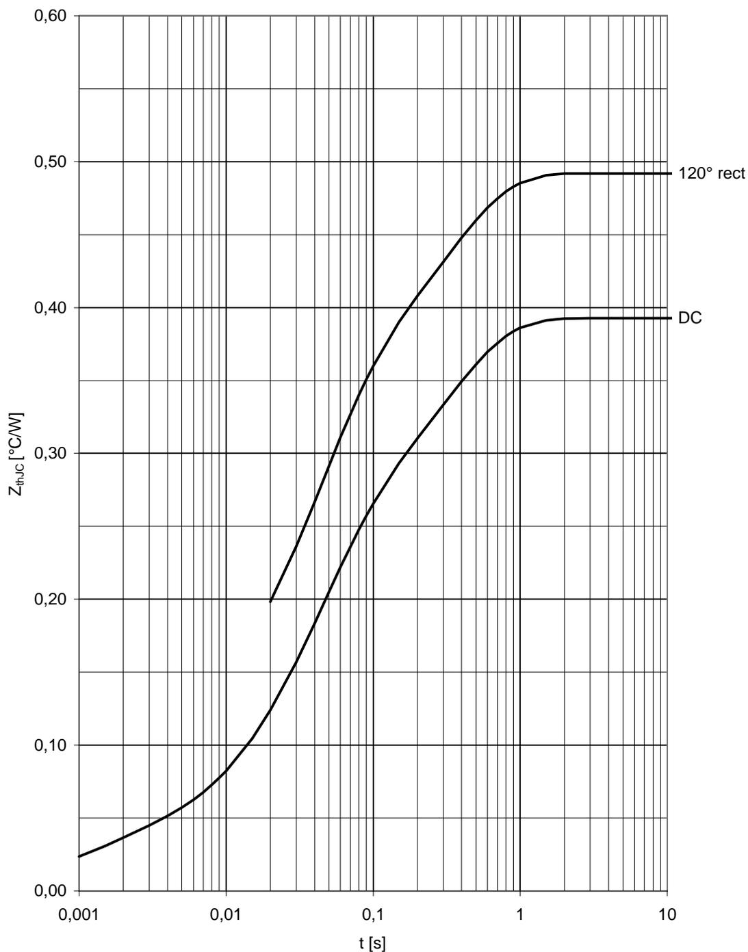
Transienter innerer Wärmewiderstand je Zweig / Transient thermal impedance per arm,  $Z_{thJC} = f(t)$
